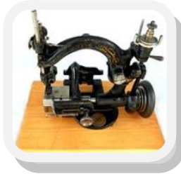
A twisted chain stitch sewing machine for making straw hats from plaited straw (C1880).
